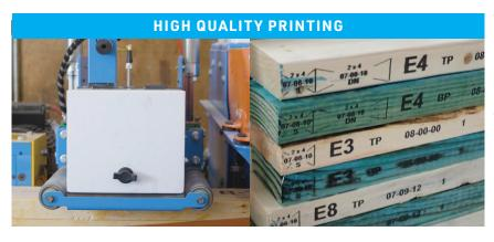
The plate layout edge printer allows for customizable printing on lumber, including a feature to print a BOM on the bottom face, enhancing assembly efficiency and accuracy without paper instructions. Plus, the part ID remains visible on stacked lumber, ready for job site delivery.
