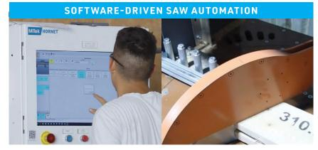
The up-cut saw, integrated with MiTek software, enables automatic cutting of top and bottom plates in one stroke. It features a fully automated infeed lumber conveyor for continuous cutting, with an outfeed sweeper for automatic removal of cut pieces.
