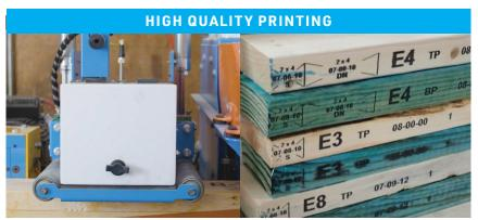
The plate layout edge printer allows for customizable printing on lumber, including a feature to print a BOM on the bottom face, enhancing assembly efficiency and accuracy without paper instructions. Plus, the part ID remains visible on stacked lumber, ready for job site delivery.
