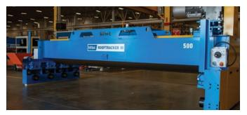
**RoofTracker III™** A high-volume roof truss roller gantry that presses the top and bottom plates in a single pass.
