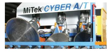
**Cyber A/T**<sup>®</sup> A versatile, computer-controlled component saw with fully powered features and options for high-speed batch-cutting.
