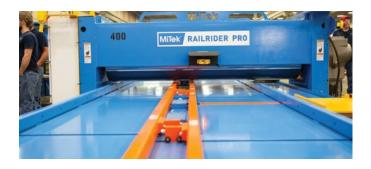
RailRider Pro® A high-volume throughput in floor truss assembly, ensuring a full plate embedment each pass.
